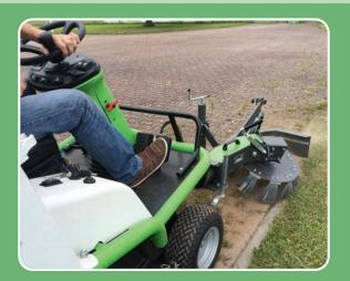
This accessory also gives more versatility of the machine by expanding its accessories range. The wire brush is assembled and disassembled easily at the front of the machine, without changes to be made in advance. Other accessories available include a mechanical spreader, sprayer, blower, sweepers, and side brush.
